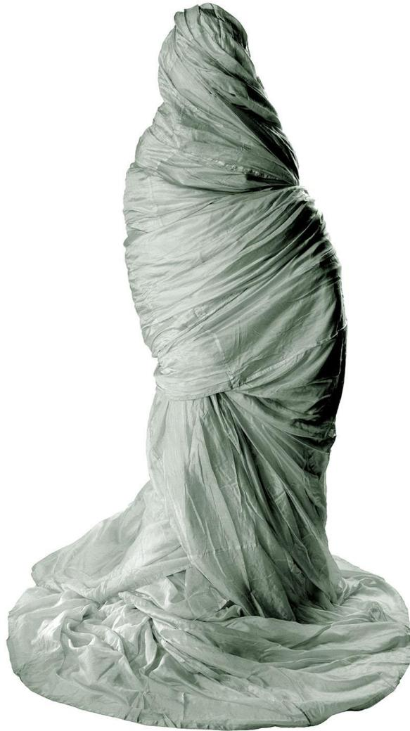
Tiny Broadwick said that unlike modern parachutes, which are shaped from bias strips to give them the strength to withstand jumps from speeding aircraft without tearing, this parachute is shaped from straight pieces of material. This back-pack parachute was used for exhibition jumps in the early-1900s. Photo by Carolyn Russo, National Air and Space Museum
