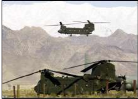
Two Chinook CH-47s in action in the war against terrorism in Afghanistan. The Chinook evolved from Piasecki's ground-breaking tandem rotor designs of the 1940s and 1950s.
